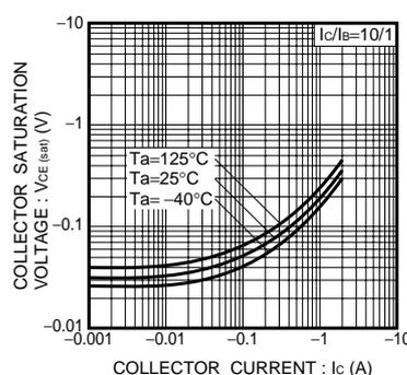
Fig.5 Collector-Emitter Saturation Voltage vs. Collector Current (I)
