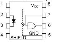
1:NC 2:ANODE **3:CATHODE** 4:N.C. 5:GND 6:V<sub>0</sub>(OUTPUT)
