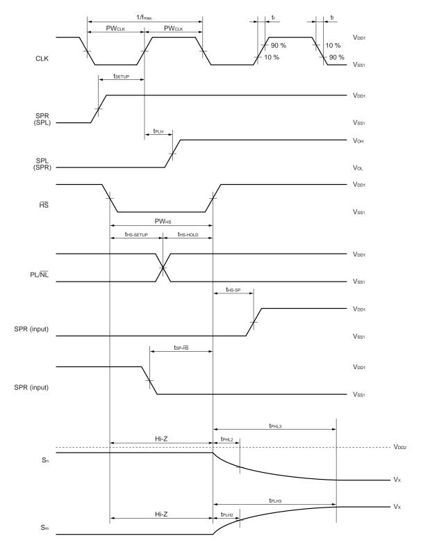
Vx refers to the final output voltage, tplh2 and tphl2 refer to the time required to an output precision level of 10 % (0.1 Vx); and tplh3 and tphl3 refer to the time required to reach an output precision level of 6 bits.
