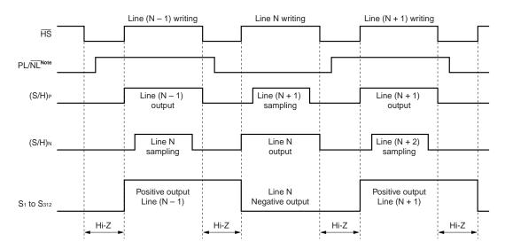
**Note**  $PL/\overline{NL} = H$ ; input negative analog display signal.  $PL/\overline{NL} = L$ ; input positive analog display signal.
