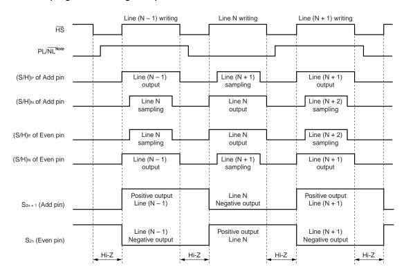
**Note** Odd number pin  $PL/\overline{NL} = H$ ; input negative analog display signal.
