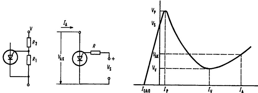
$$R_g = \frac{R_1 \cdot R_2}{R_1 + R_2}$$
