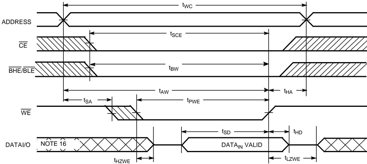
**Write Cycle No. 4 ( $\overline{BHE/BL\overline{E}}$  Controlled,  $\overline{OE}$  LOW)<sup>[15]</sup>**
