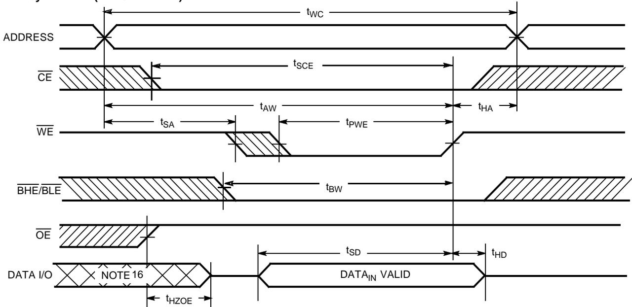
**Write Cycle No. 2 ( $\overline{CE}$  Controlled)** <sup>[10, 14, 15]</sup>
