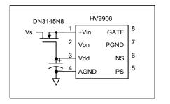
This method limits the +V<sub>IN</sub> voltage to V<sub>DD</sub> + V<sub>GS(OFF)</sub> of the depletion MOSFET for all input voltages and in fact raises the maximum allowable peak input voltage to the breakdown voltage rating of the depletion MOSFET. The worst-case power dissipation in the HV9906 is now given by the equation
