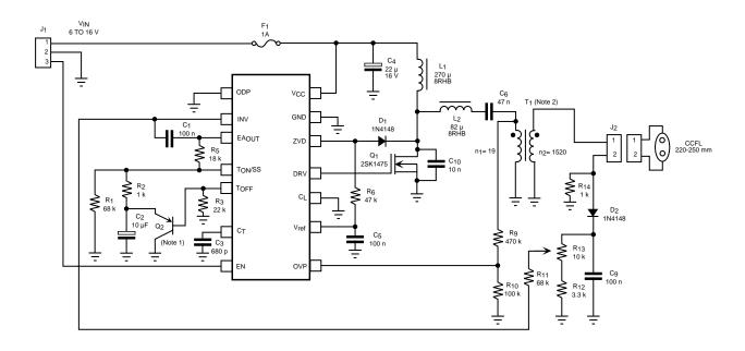
$\begin{array}{ll} \mbox{Gen. Note:} & \mbox{Q}_2 \mbox{ is not required if Q}_1 \mbox{ is an avalanche rated FET} \\ \mbox{Gen. Note:} & \mbox{Part \#CTX01-13154 (Call Toko Technical Support (719) 528-2200).} \end{array}$
