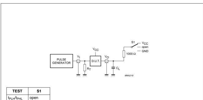
Fig.9 Load circuit for switching times.
