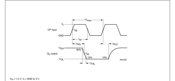
Fig.6 The clock (CP) to output (Q<sub>n</sub>) propagation delays, the clock pulse width, the output transition times and maximum clock pulse frequency.
