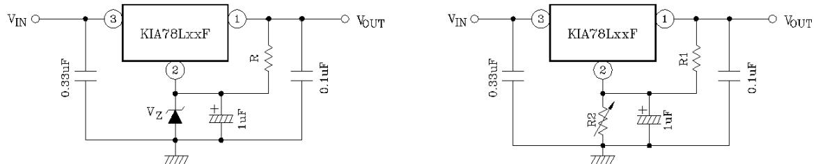
$V_{OUT} = V_Z + V_{OUT}$  (of IC)
