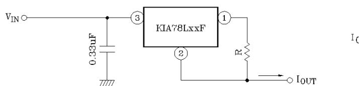
$$I_{OUT} = \frac{V_{OUT}}{R} + I_B$$
