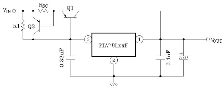
$$R_{SC} = \frac{V_{BE2}}{I_{SC}}$$
