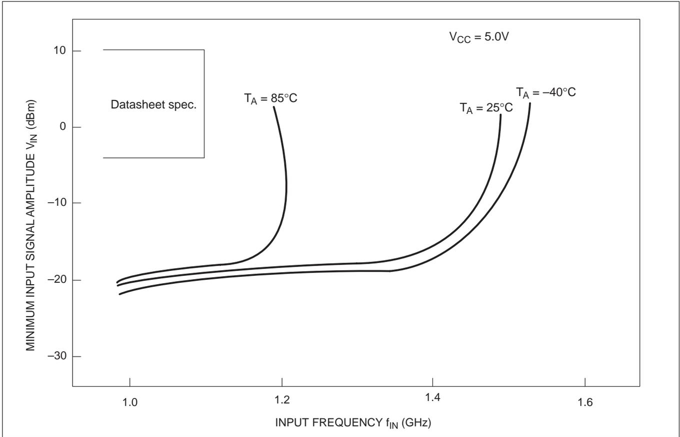
Figure 3. Input Signal Amplitude vs. Input Frequency
