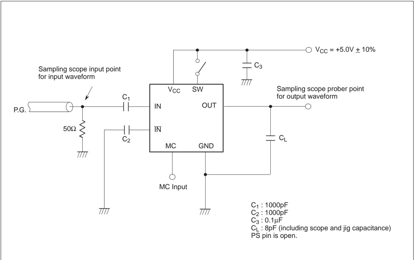
Figure 2. Test Circuit
