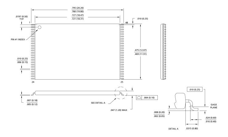
**NOTE:** 1. All dimensions in inches (millimeters) MAX or typical where noted.
