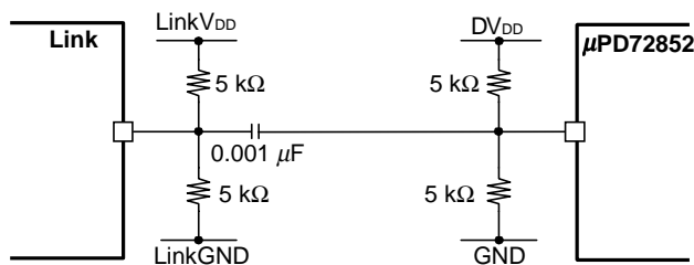
(e) SCLK Isolation Barrier Circuit
