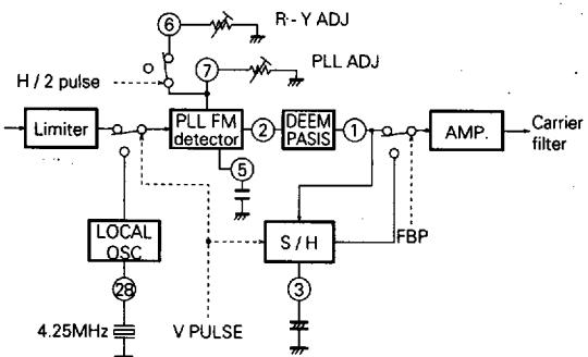
The R-Y black level is adjusted to the B-Y black level by varying the external resistor at pin 6.
