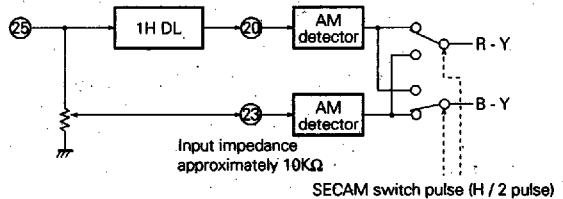
Pin 25 outputs the chroma signal, and the direct signal is input to pin 23, the delayed signal to pin 20. After each signal is AM detected, R-Y and B-Y are obtained by switching between detector outputs every 1H.
