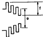
**Note15.** Set VEXT3 to 5.7V. Change VEXT1 so that the average voltage on pin ⑩ becomes 7.2V. At this time, measure the distortion at pins ⑩, ⑭.
