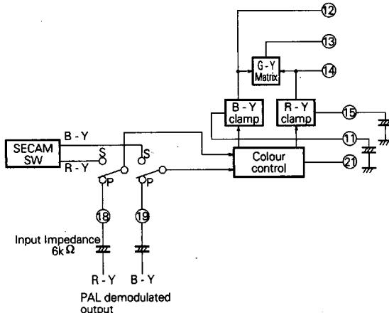
The R-Y signal and B-Y signal pass through this system switch and are routed to the colour control circuit, where clamping takes place; G-Y is obtained.
