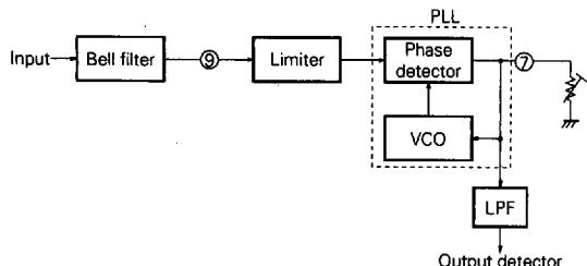
The PLL consists of an emitter coupled multivibrator VCO and double balanced multiplier. The output of the VCO is multiplied by the limiter output, and this is fed back to the VCO. When the PLL is locked on to the input of the FM detector, the output of the PLL becomes the phase detector output, which is passed on to the LPF.
