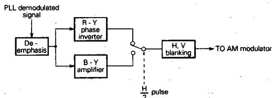
The signal obtained by the PLL FM demodulator is input to the amplifier circuit after de-emphasis by external parts. Then R-Y is phase inverted, and the gain ratio of R-Y and B-Y is
