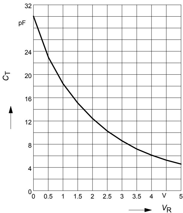
**Normalized diode capacitance**
