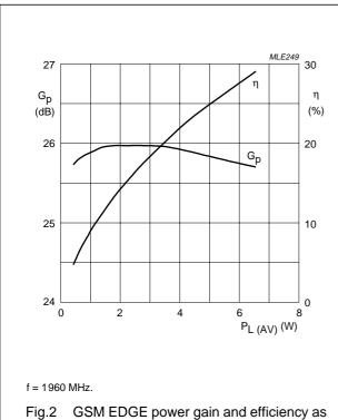
Fig.2 GSM EDGE power gain and efficiency as functions of load power; typical values.
