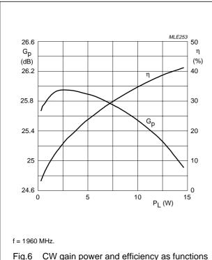
Fig.6 CW gain power and efficiency as functions of load power; typical values.
