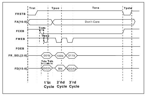
Figure 12.11 Timing Diagram of Erase
