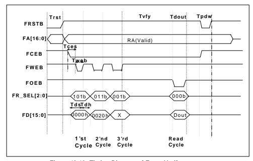
Figure 12.13 Timing Diagram of Erase Verify
