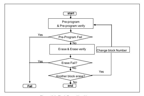
Figure 12.8 Flash Erase Algorithm
