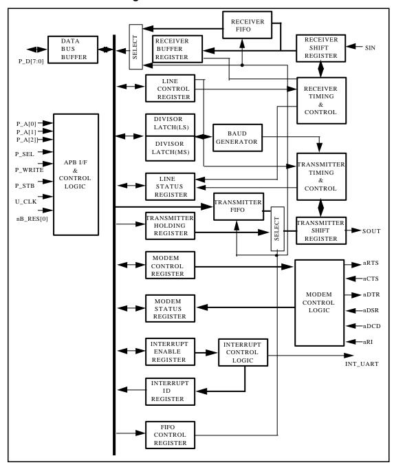
Figure 9.2 Internal UART Diagram
