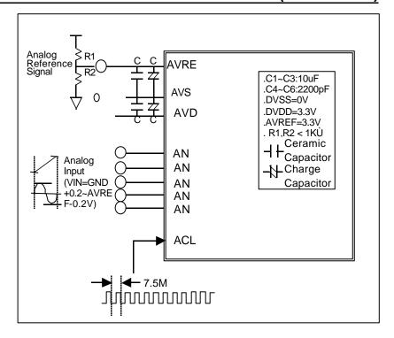
Figure 13.3 Example of Analog Input Circuit
