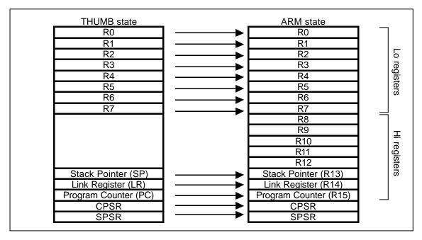
Figure 2.6 Mapping of THUMB state registers onto ARM state registers.
