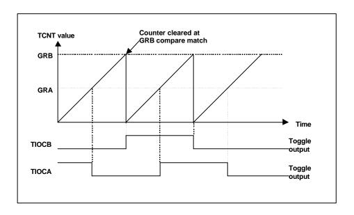
Figure 8.5 Example of Toggle Output
