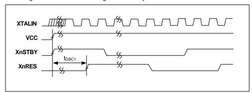
Figure 14.1 The settling time of the crystal oscillator
