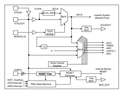
Figure 5.1 PMU Block Diagram
