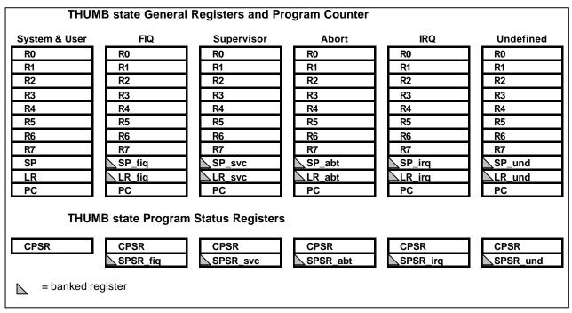
Figure 2.5 Register Organization in THUMB state
