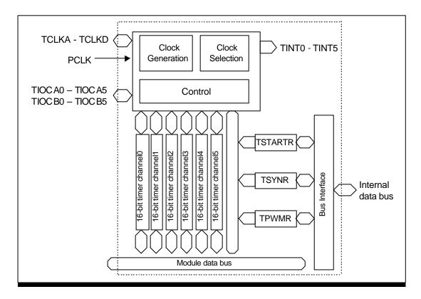
Figure 8.1 General-purpose Timer Unit Module Block Diagram
