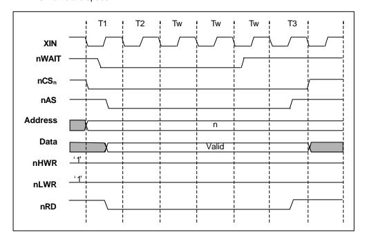
Figure 3.17 Example of Wait State Insertion Timing.
