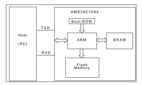
Figure 12.2 System Configuration When Using On-Board Boot Mode
