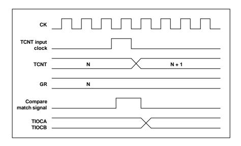
Figure 8.6 Compare Match Signal Output Timing
