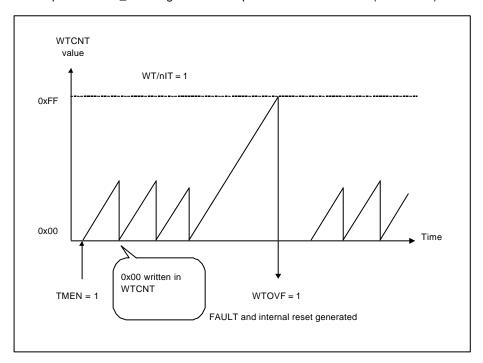
Figure 7.2 Operation in the Watchdog Timer Mode
