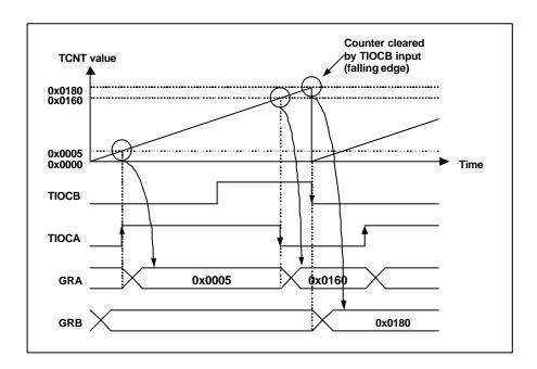
Figure 8.7 Input Capture Operation
