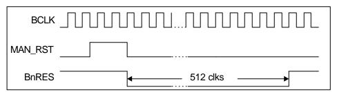
Figure 5.5 Soft Reset (from WDT) Timing Diagram
