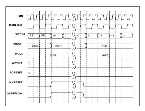
Figure 7.7 Interrupt Clear in the Watchdog Timer Mode with Manual Reset
