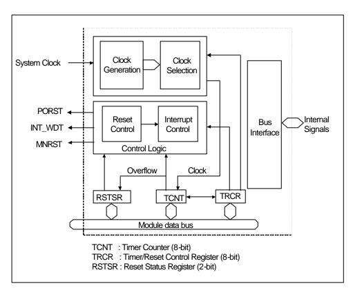
Figure 7.1 Watchdog Timer Module Block Diagram
