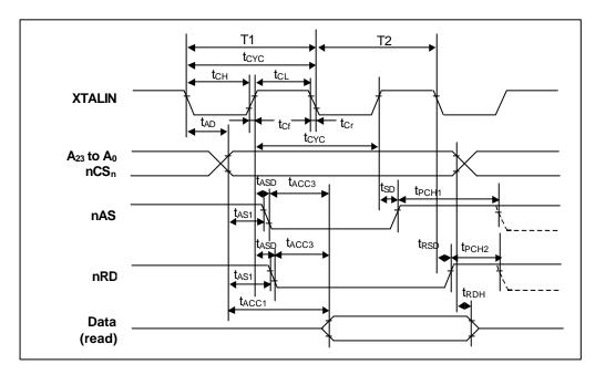
Figure 14.4 The Read Timing Diagram of the Bus Controller
