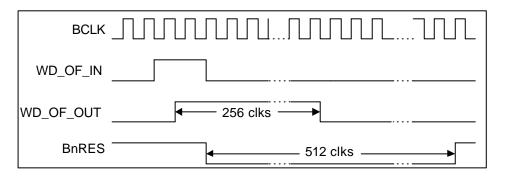
Figure 5.4 Watch Dog Timer Overflow Timing Diagram
