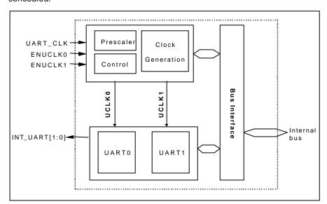
Figure 9.1 TOP BLOCK Diagram
