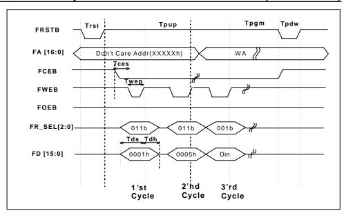
Figure 12.10 Timing Diagram of Pre-Program/Program
