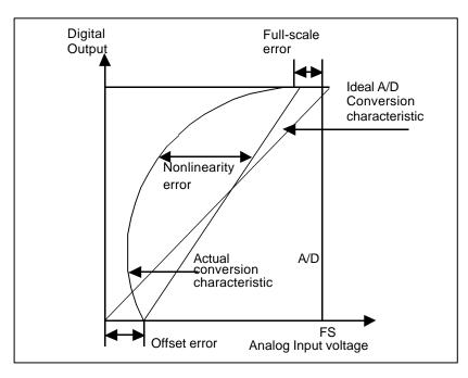
Figure 13.4 A/D Converter Accuracy Definitions (1)
