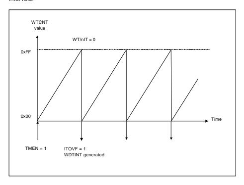
Figure 7.3 Operation in the Interval Timer Mode
