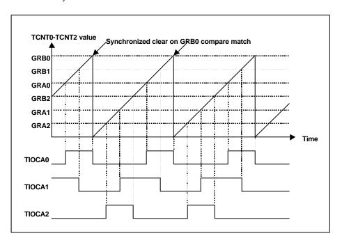
Figure 8.8 Synchronized Operation Example
