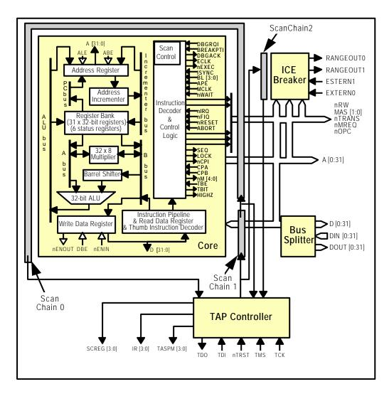
Figure 2.1 ARM7TDMI Core Block Diagram
