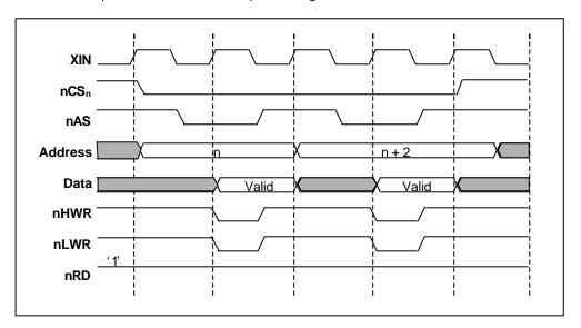
Figure 3.5 Bus Control Signal Write Timing for 16-Bit, 1-Wait (Word Access)
