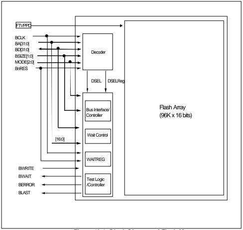
Figure 12.1 Block Diagram of Flash Memory
