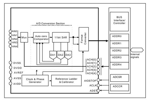
Figure 13.1 Block Diagram of A/D Converter
