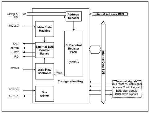
Figure 3.1 Block Diagram of the Bus Controller
