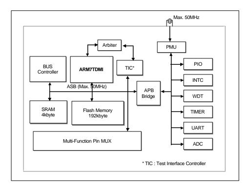
Figure 1.2 HMS39C7092 Block Diagram
