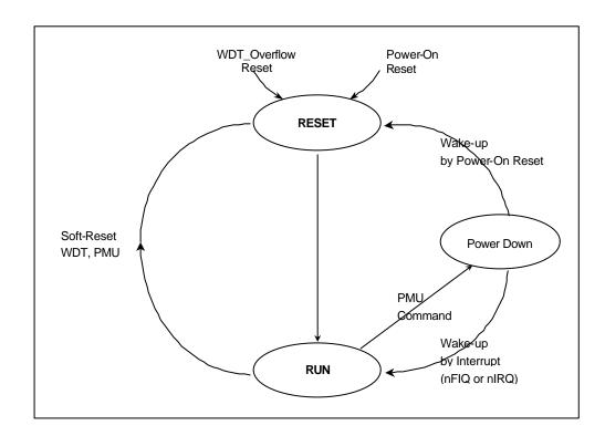
Figure 5.2 Reset and Power Management State Machine.
