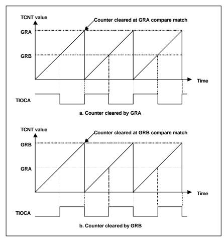
Figure 8.9 PWM Mode Operation Example 1
