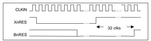
Figure 5.3 Power on Reset Timing Diagram
