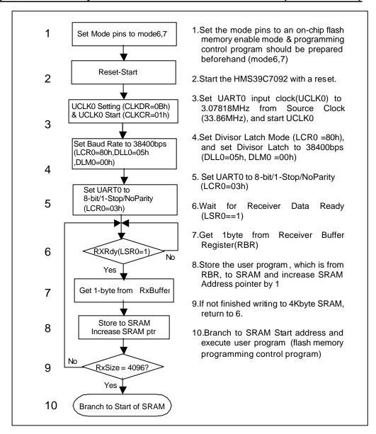
Figure 12.3 Boot Mode Execution Procedure
