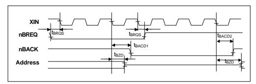
Figure 14.6 Bus Release Mode Timing
