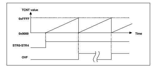
Figure 8.2 Free-Running Counter Operation
