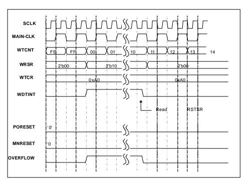
Figure 7.4 Interrupt Clear in the Interval Timer Mode
