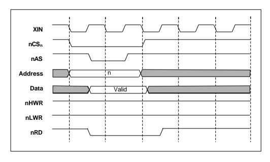
Figure 3.10 Bus Control Signal Read Timing for 16-Bit, 1-Wait (Byte Access)
