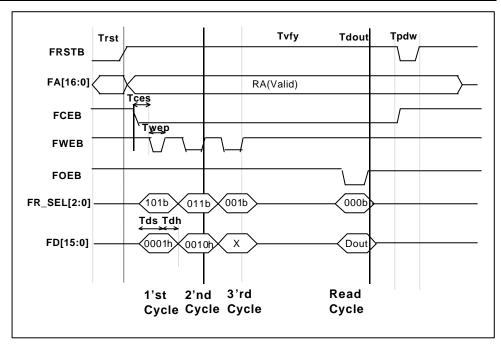
Figure 12.12 Timing Diagram of Pre-Program/Program Verify
