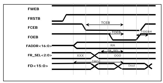
Figure 12.9 Timing Diagram of Read
