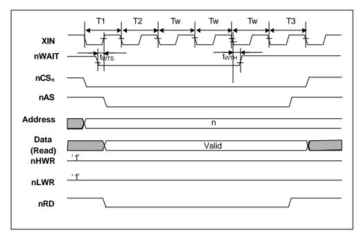
Figure 14.5 Basic Bus Cycle with External Wait State
