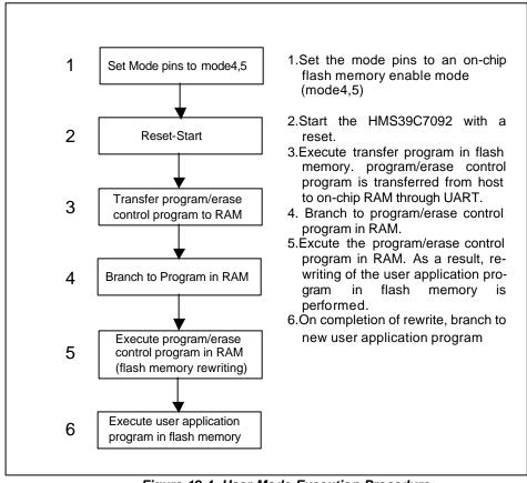
Figure 12.4 User Mode Execution Procedure
