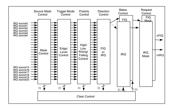
Figure 6.1 Interrupt Control Flow Diagram
