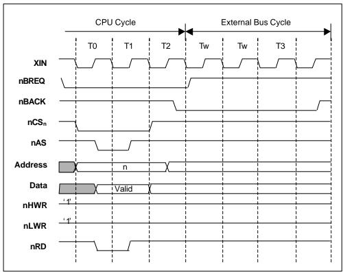
Figure 3.18 Example of External Bus Master Operation
