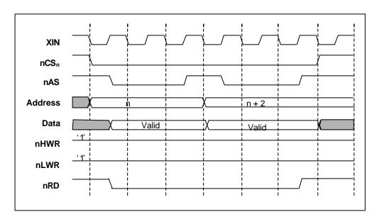
Figure 3.12 Bus Control Signal Read Timing for 16-Bit, 2-Wait (Word Access)
