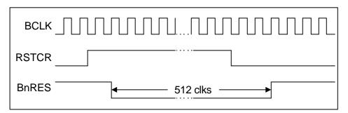
Figure 5.6 Soft Reset (from PMU) Timing Diagram
