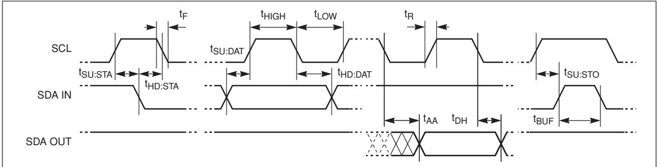
Figure 5. WP, A0, A1, V<sub>P</sub> Pin Timing
