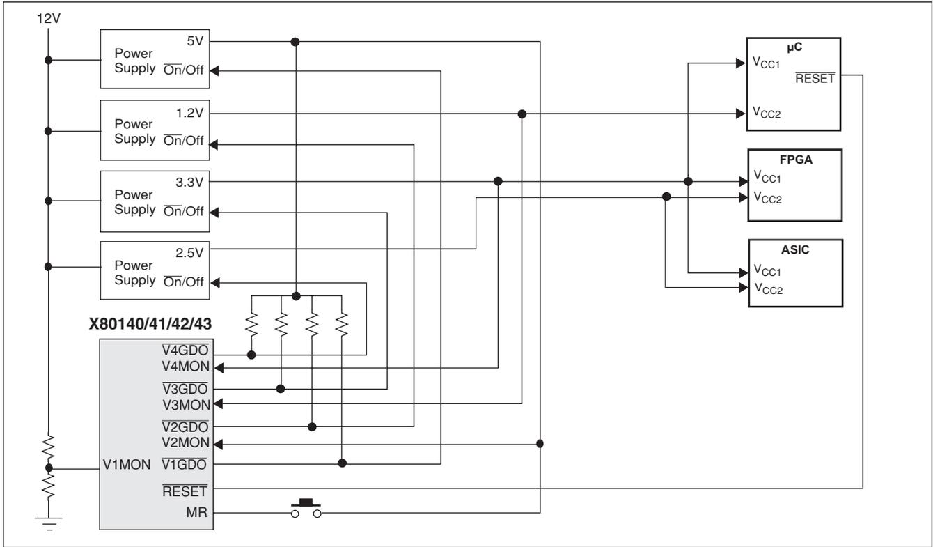
Figure 10. Relay Sequencing of DC-DC Supplies. (Timing)
