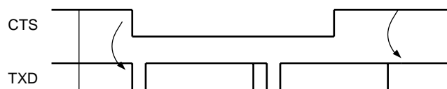
Figure 189. Transmitter Behavior when Operating with Hardware Handshaking
