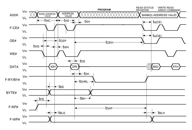
M6MGB/T160S2BVP 16,777,216-BIT (1,048,576 -WORD BY 16-BIT / 2,097,152-WORD BY 8-BIT) CMOS
