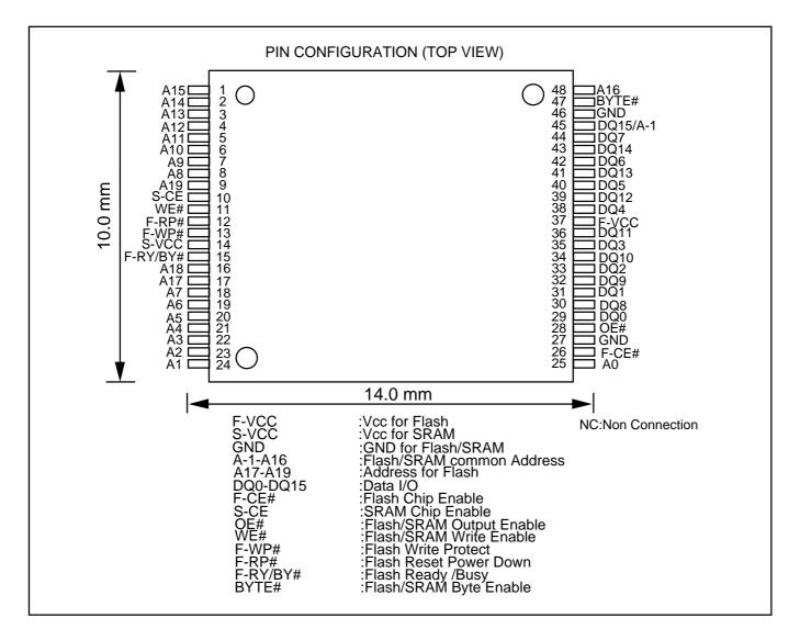
M6MGB/T160S2BVP 16,777,216-BIT (1,048,576 -WORD BY 16-BIT / 2,097,152-WORD BY 8-BIT) CMOS 3.3V-ONLY FLASH MEMORY & 2,097,152-BIT (131,072-WORD BY 16-BIT / 262,144-WORD BY 8-BIT) CMOS SRAM Stacked-MCP (Multi Chip Package)
