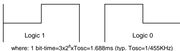
Figure 2: Biphase Code Transmission Technique
