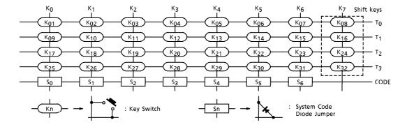
K<sub>08</sub>, 16, 24 and 32 (the shift key) keys can be pushed simultaneously with other keys (the normal keys).
