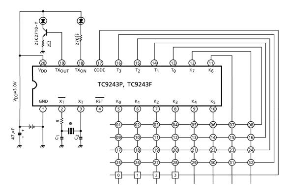
% Ceramic Oscillator CSB455E (Murata Seisakusho)  $C_1=C_2=100 pF$   $R=6.8k\Omega$  FCR455K3 (TDK)  $C_1=C_2=220 pF$   $R=2.2k\Omega$  or equivalent
