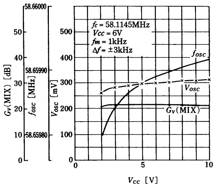
**Signal Meter-Supply Voltage Characteristics**
