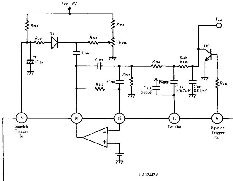
Note: Connect C119 to Vcc line as near to pin 13 as possible.
