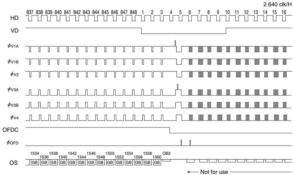
\* Do not use the field signals immediately after frame accumulation mode is transferred to field accumulation mode for monitoring image.
