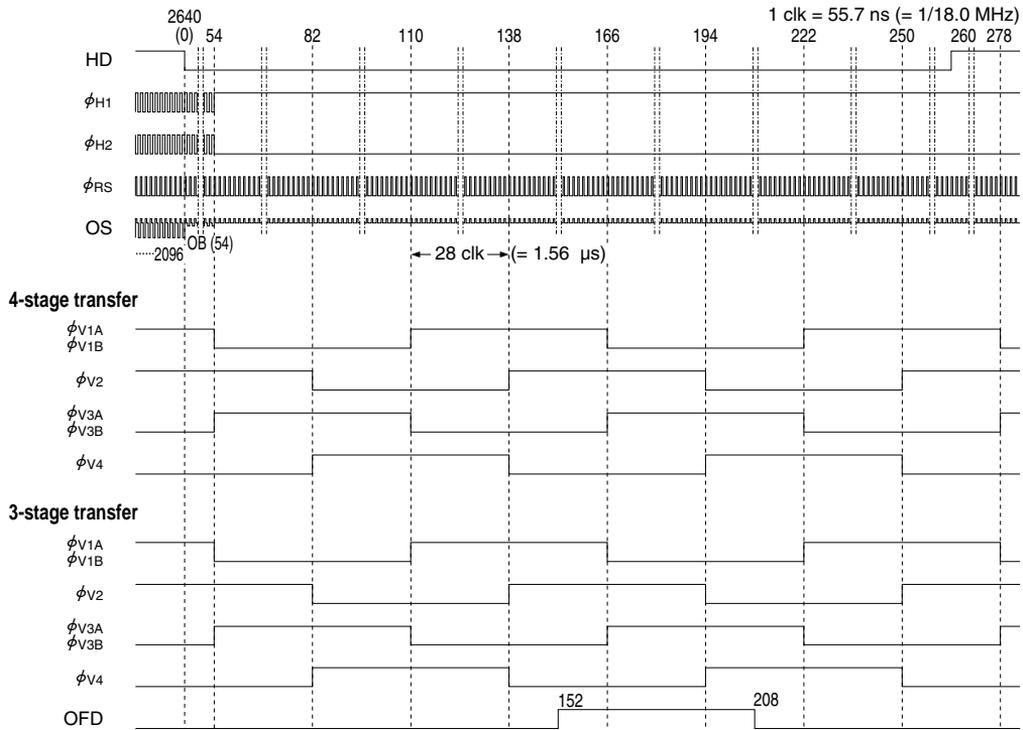
\* Keep over 1.56  $\mu$ s when vertical transfer clock pulse is overlapping.
