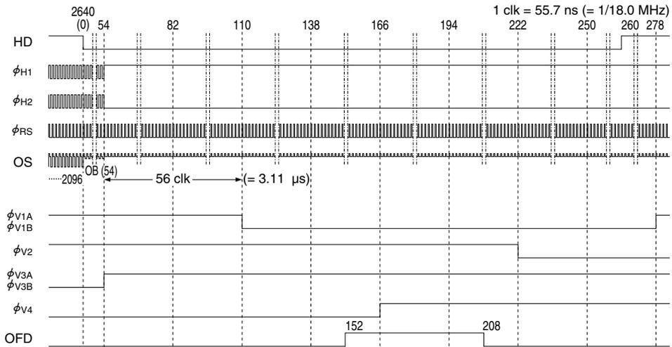
\* Keep over 3.11  $\mu$ s when vertical clock pulse is overlapping.
