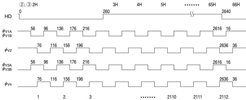
\* Keep over 1.56 μs when vertical transfer clock pulse of charge swept transfer is overlapping.
