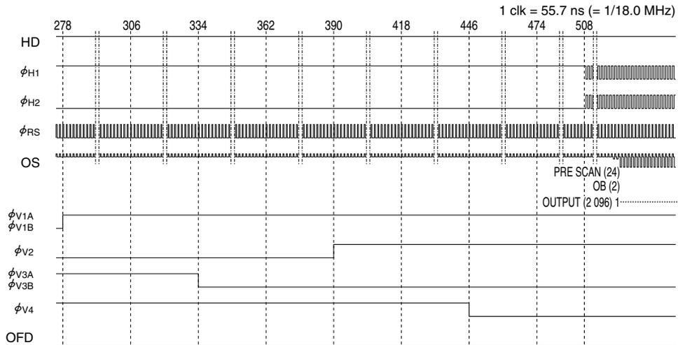
\* Keep over 3.11  $\mu$ s when vertical transfer clock pulse is overlapping.
