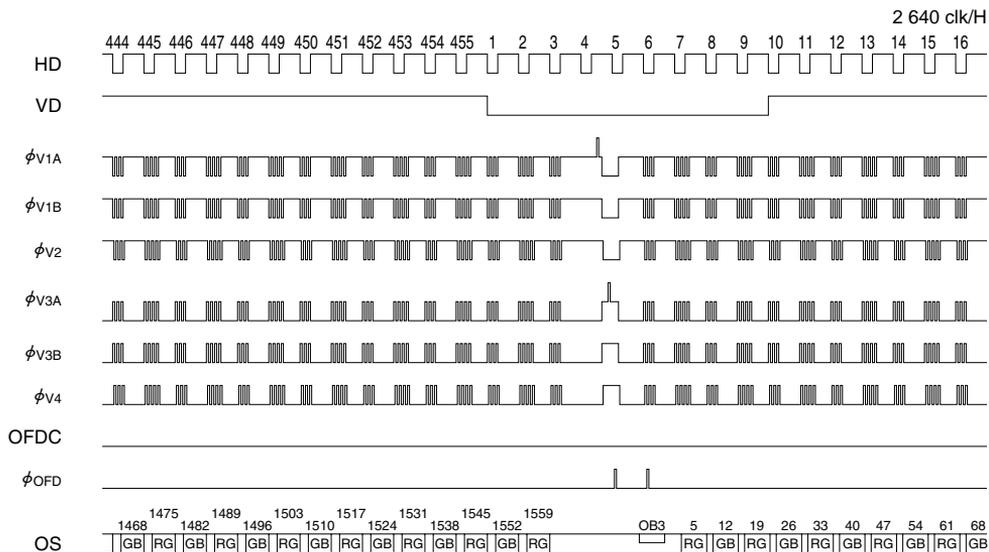
② VERTICAL TRANSFER TIMING [AT FIRST FRAME ACCUMULATION MODE]
