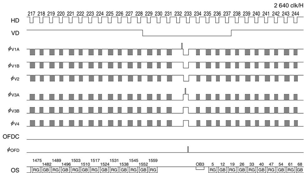
①\* VERTICAL TRANSFER TIMING [FIELD ACCUMULATION MODE]
