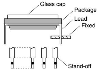
3) When mounting the package on the housing, be sure that the package is not bent.
