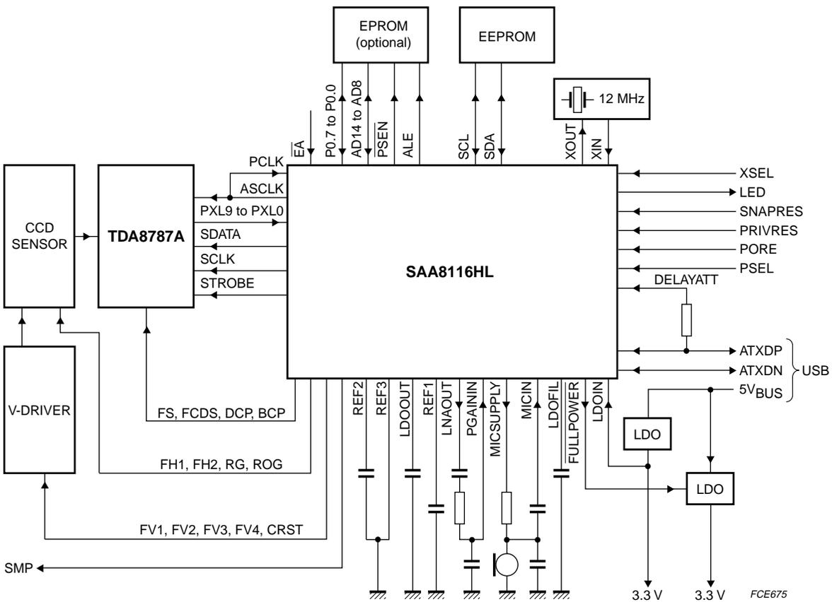
Fig.3 CCD sensor application.
