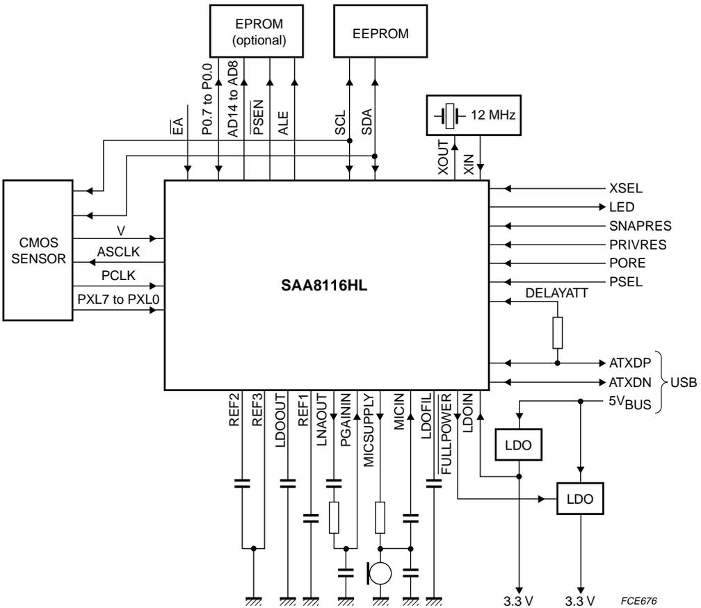
Fig.4 CMOS sensor application.
