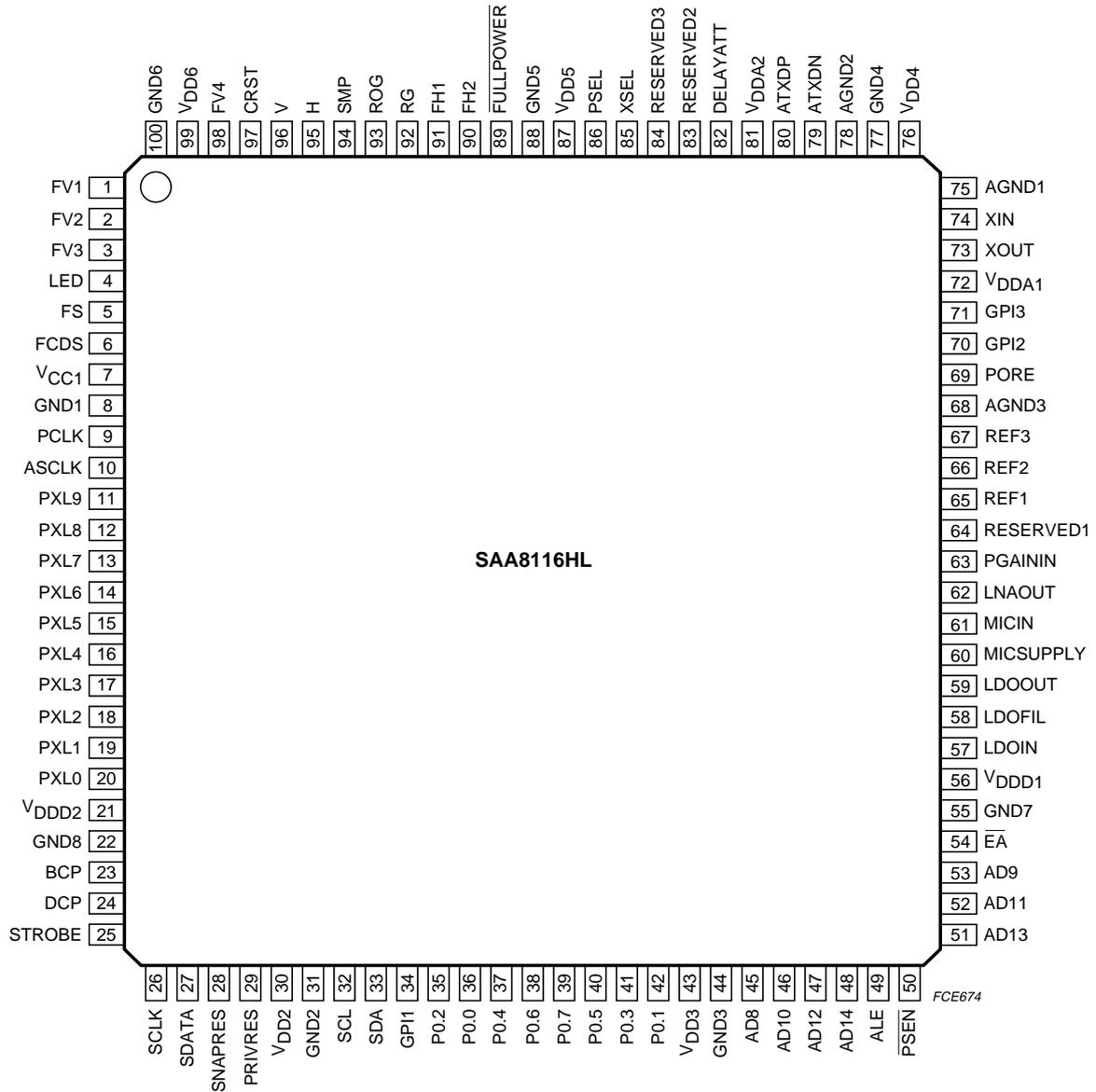
Fig.2 Pin configuration.
