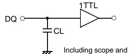
Fig.1 Output load
