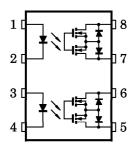
1, 3: ANODE 2, 4: CATHODE 5: DRAIN D1 6: DRAIN D2 7: DRAIN D3
