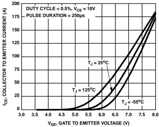
Figure 13. Transfer Characteristic
