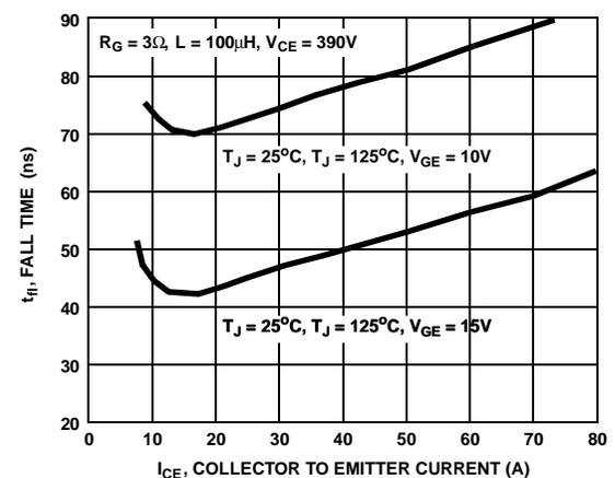
Figure 12. Fall Time vs Collector to Emitter Current
