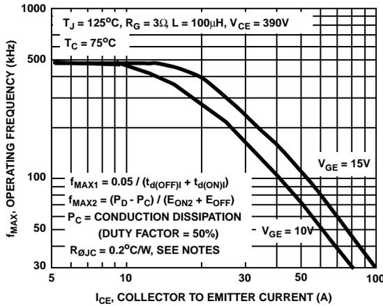
Figure 3. Operating Frequency vs Collector to Emitter Current
