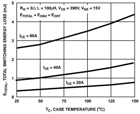
Figure 15. Total Switching Loss vs Case Temperature
