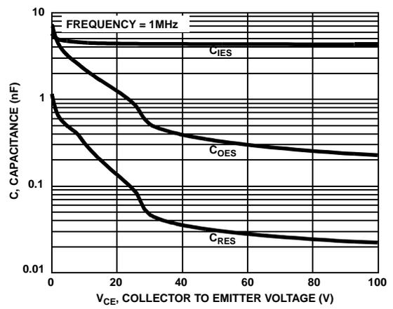
Figure 17. Capacitance vs Collector to Emitter Voltage
