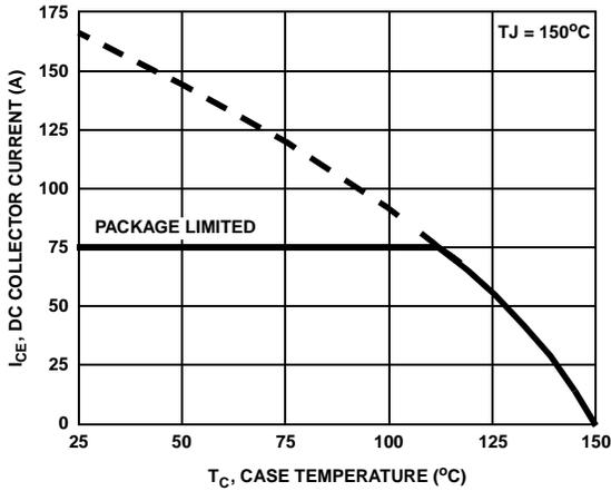
Figure 1. DC Collector Current vs Case Temperature
