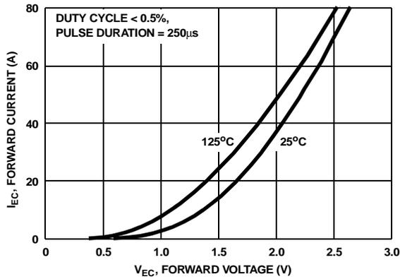
**Figure 19. Diode Forward Current vs Forward Voltage Drop**
