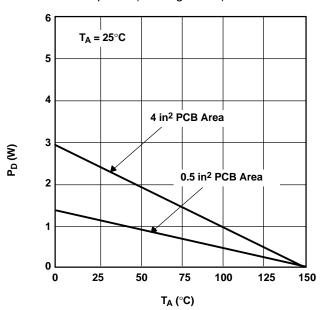
Figure 27. SOT223 Maximum Power Dissipation vs Ambient Temperature
