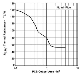
Figure 26. SOT223 Thermal Resistance vs PCB Copper Area
