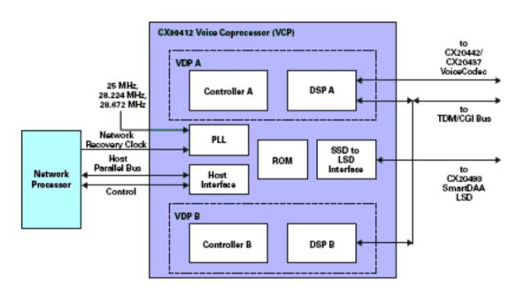
CX90412 Voice Coprocessor (VCP) Simplified Interface System Block Diagram
