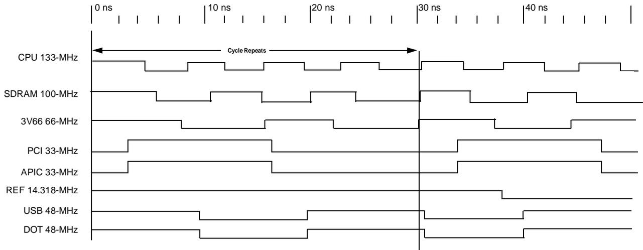
**Figure 4. Group Offset Waveforms (133-MHz CPU/100-MHz SDRAM)**
