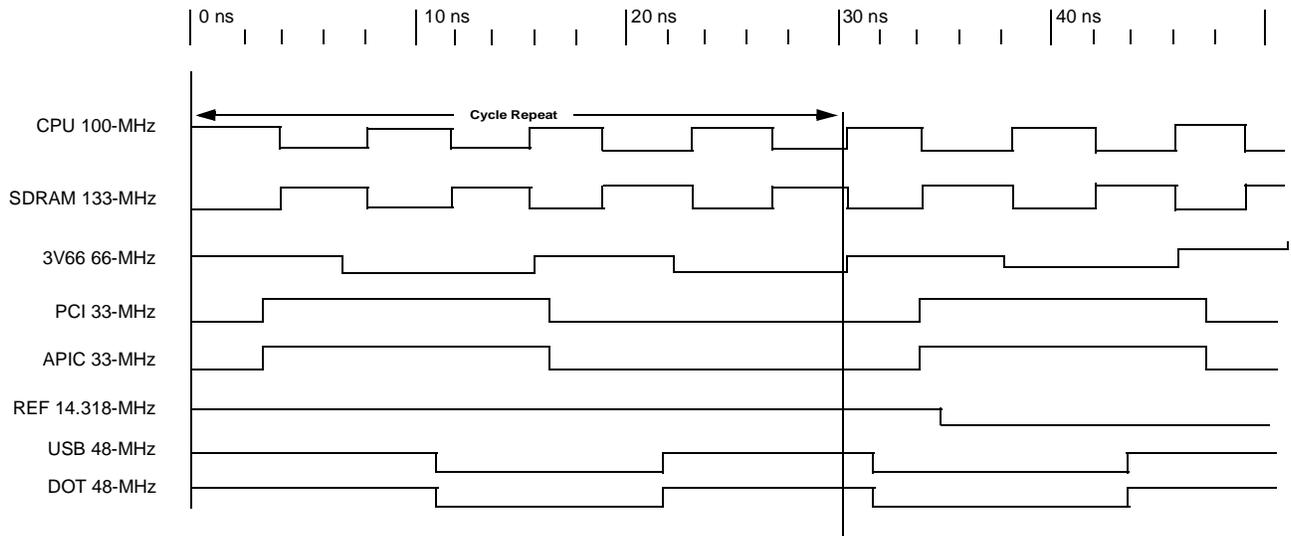
**Figure 5. Group Offset Waveform (133-MHz CPU/133-MHz SDRAM)**
