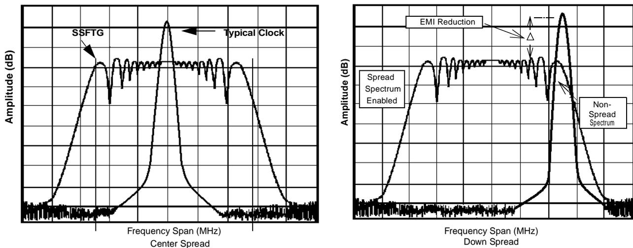
**Figure 7. Clock Harmonic with and without SSCG Modulation Frequency Domain Representation**
