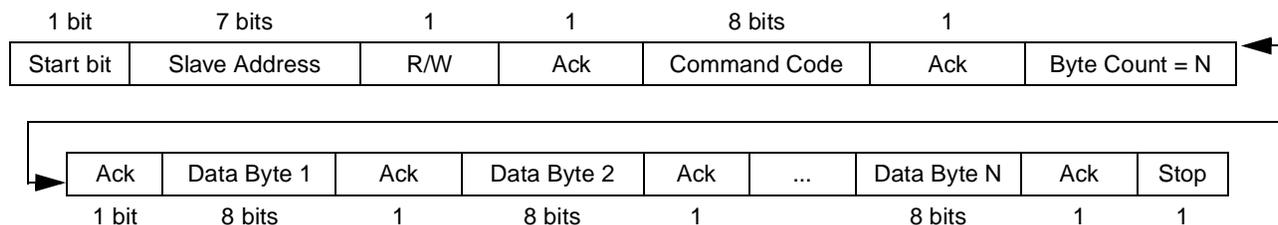
**Figure 9. An Example of a Block Write<sup>[6]</sup>**
