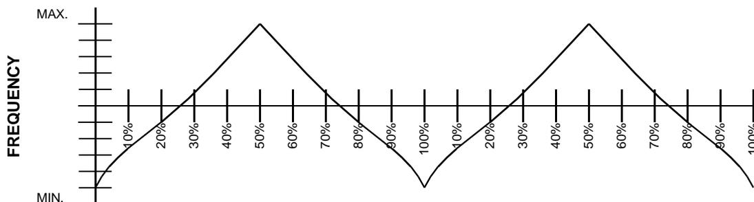
**Figure 8. Typical Modulation Profile**
