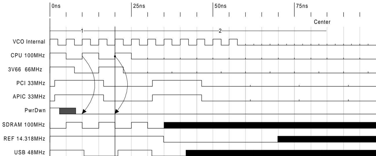
**Figure 6. W229B PWRDWN# Timing Diagram**<sup>[2, 3, 4, 5]</sup>
