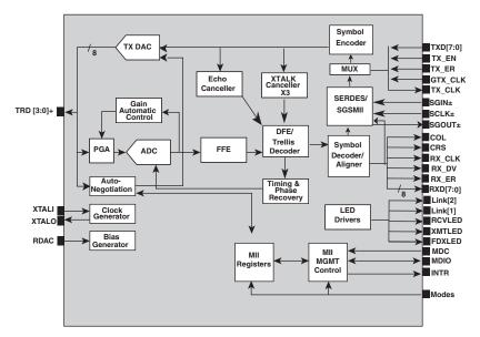
The BCM5421S is a fully integrated 10/100/1000BASE-T Gigabit Ethernet transceiver. The BCM5421S is optimized for low power and small footprint size to enable GBIC, copper, and fiber applications. By lowering system cost and reducing power dissipation by nearly 50%, the BCM5421S enables a new class of cost-effective Gigabit Ethernet equipment.
