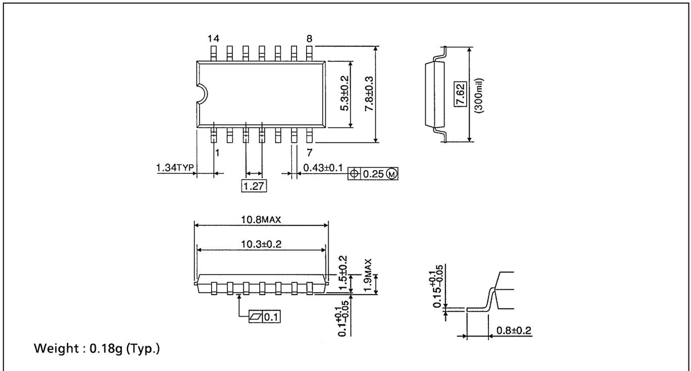
**SOP 14PIN (150mil BODY) PACKAGE DIMENSIONS (SOP14-P-150-1.27)**
