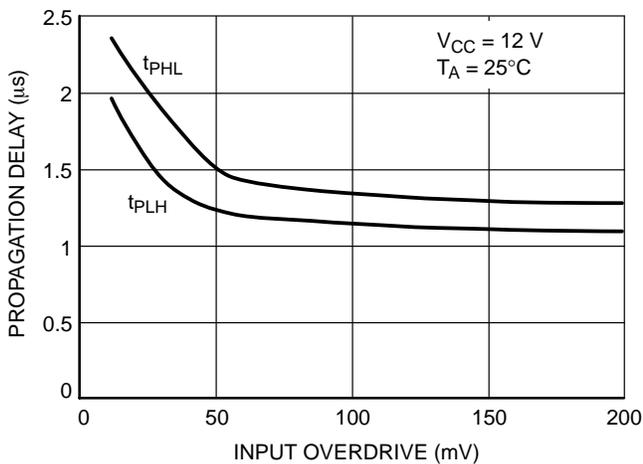
**Figure 11. NCS2300 Series Propagation Delay vs. Input Overdrive**
