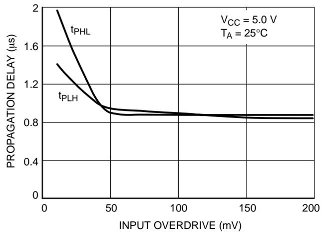
**Figure 10. NCS2300 Series Propagation Delay vs. Input Overdrive**
