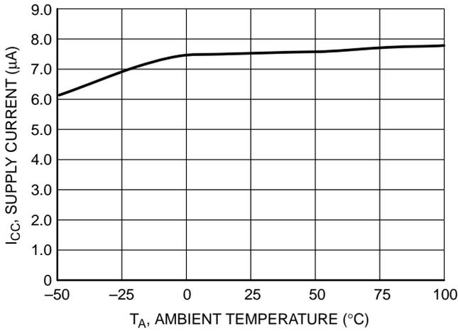
**Figure 1. NCS2300 Series Supply Current vs. Temperature**
