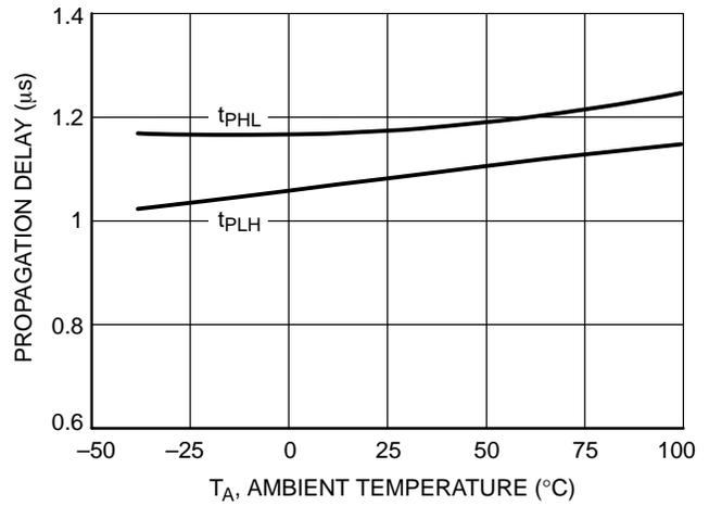
**Figure 8. NCS2300 Series Propagation Delay vs. Temperature**
