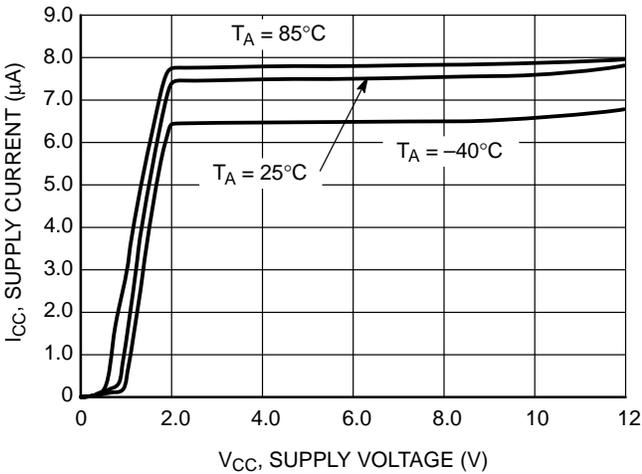
**Figure 3. NCS2300 Series Supply Current vs. Supply Voltage**
