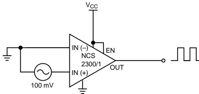
**Figure 20. Zero-Crossing Detector**
