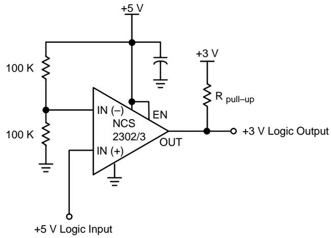
This circuit converts 5 V logic to 3 V logic. In using the NCS2202/3 allows for full 5 V logic swing without creating overvoltage on the 3 V logic input.
