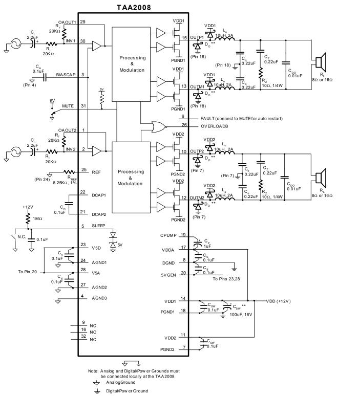
$^{**}$  For VDD voltages above 13.2V, output diodes (D $_{\rm O}$ ) should be used and the value of C $_{\rm SW}$  should be increased to 220uF. All Diodes are Motorola MBRS130T3 or equivalent.
