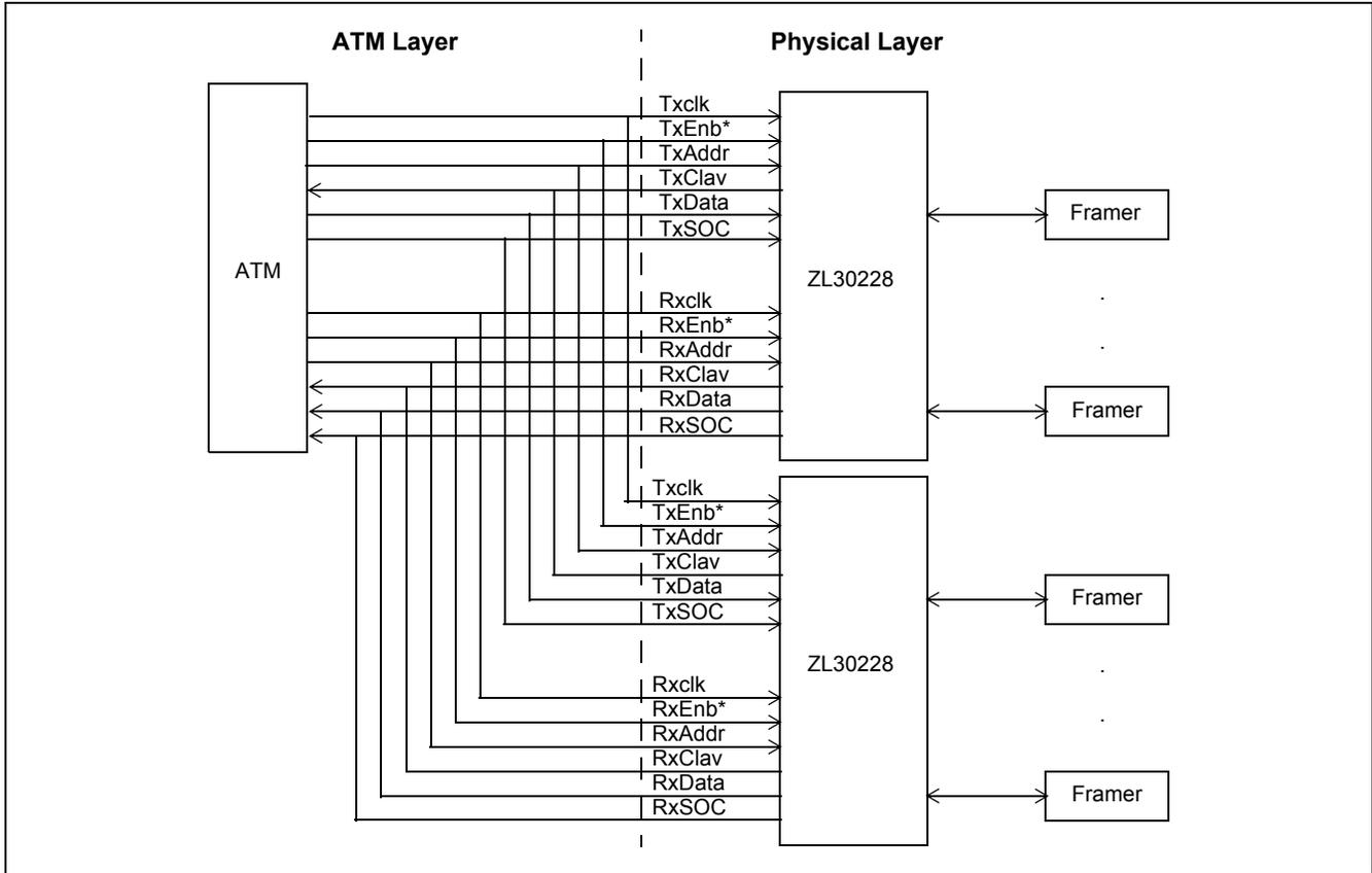
Figure 13 - ATM Interface to Multiple ZL30228s
