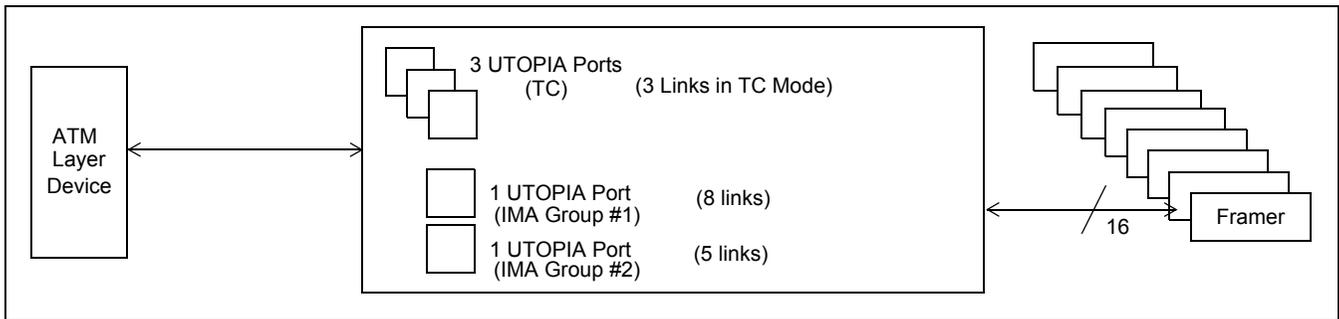
Figure 14 - ATM Mixed-Mode Interface to One ZL30228
