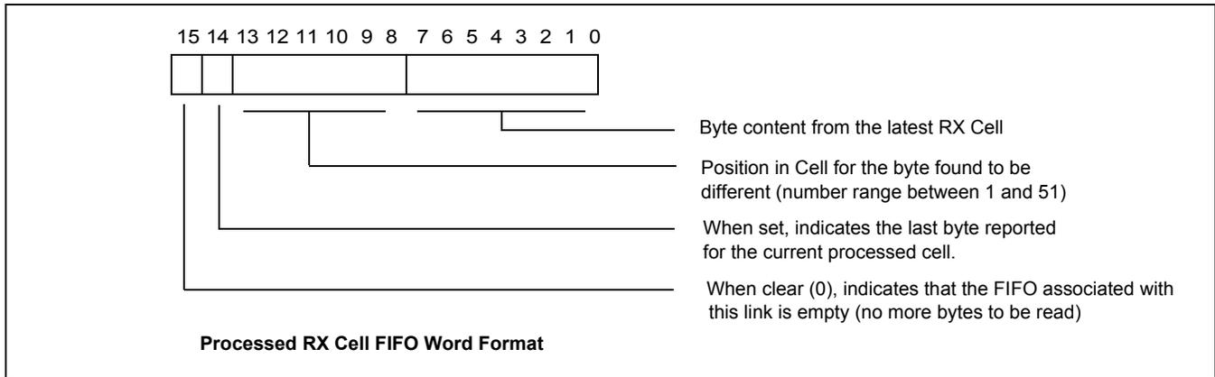
**Figure 16 - Processed RX Cell FIFO Word Format**
