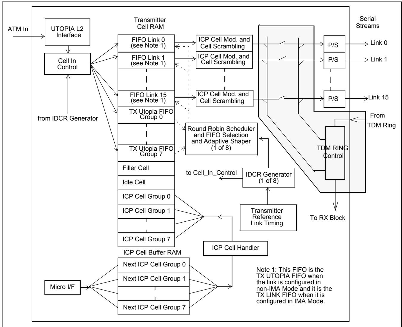
Figure 5 - ZL30228 Functional Block Diagram -Transmitter in IMA Mode
