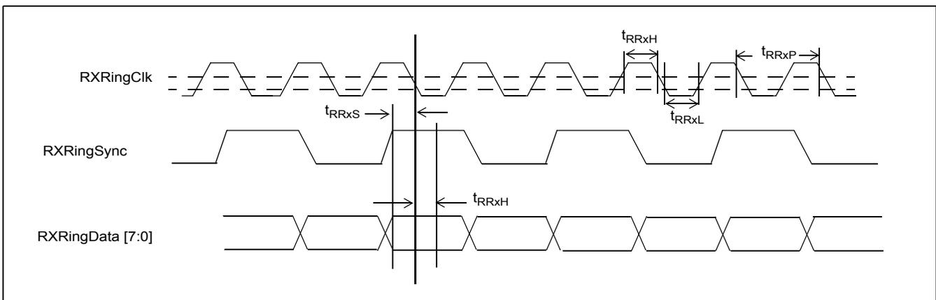
Figure 29 - TDM Ring RX Timing Diagram
