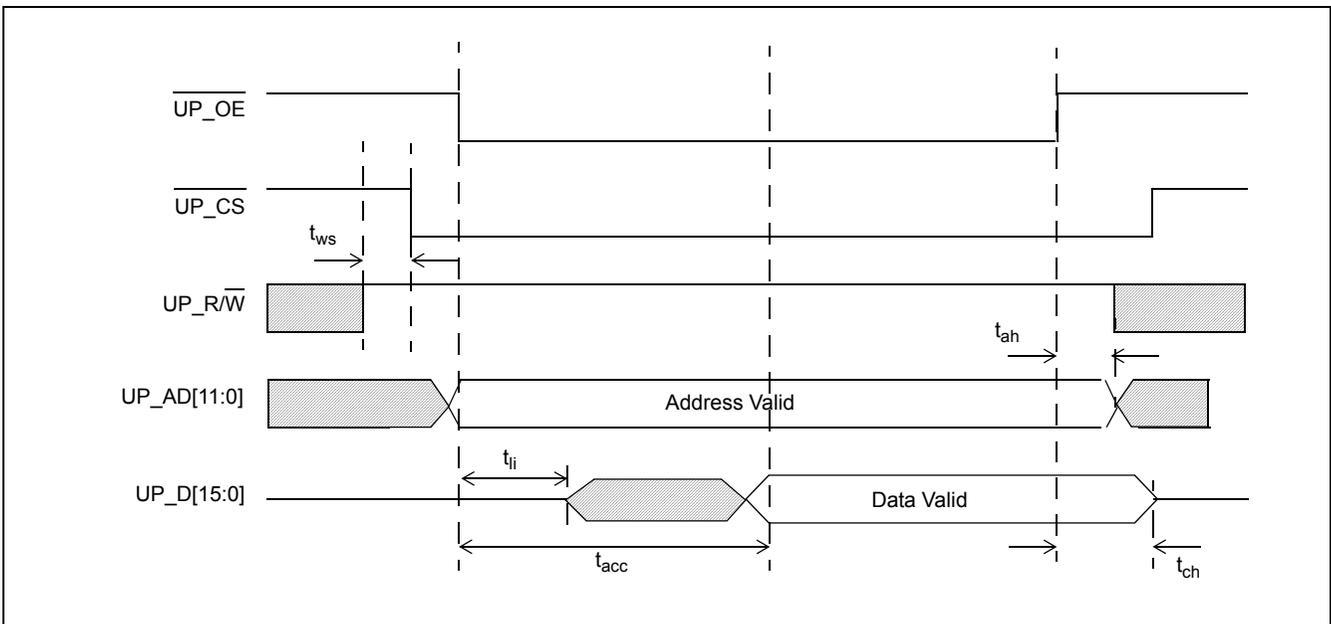
**Figure 24 - CPU Interface Intel Timing - Read Access**
