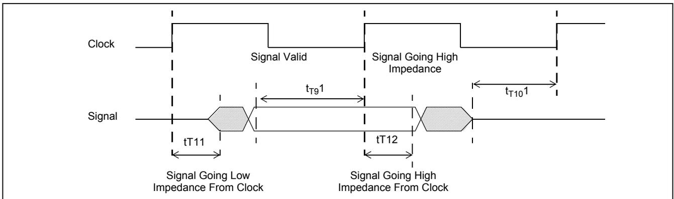
**Figure 19 - Tri-State Timing**
