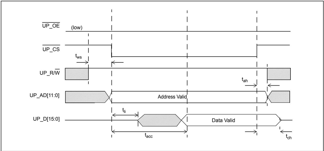
**Figure 23 - CPU Interface Motorola Timing - Read Access**
