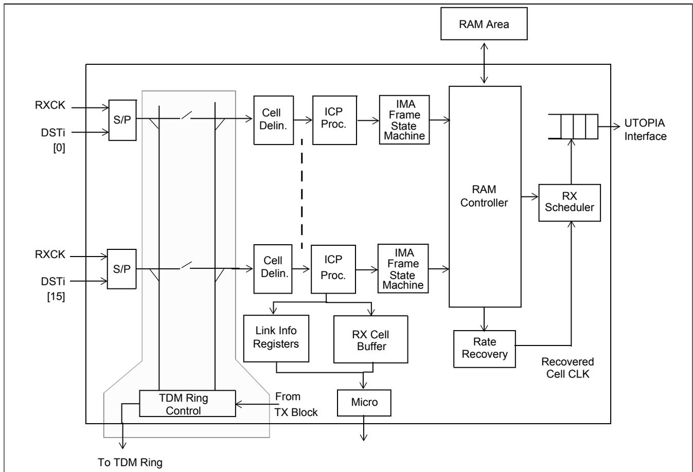
Figure 9 - ZL30228 Receiver Circuit in IMA Mode
