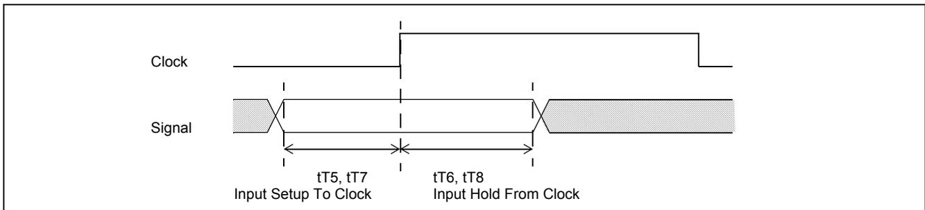
**Figure 18 - Setup and Hold Time Definition**
