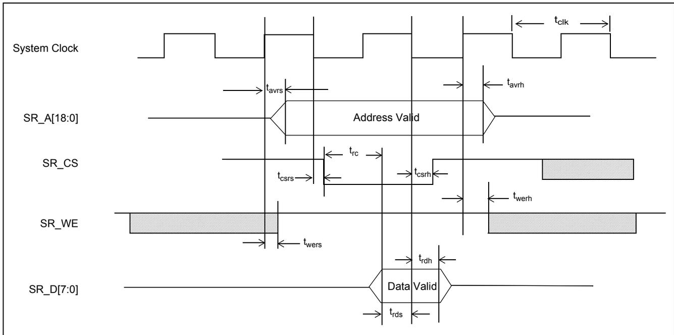
**Figure 21 - External Memory Interface Timing - Read Cycle**
