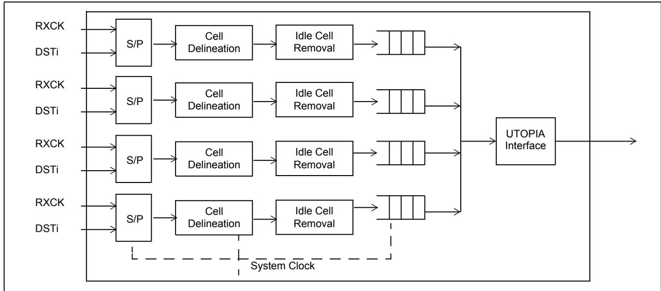
**Figure 10 - Example of TC Mode Operation
