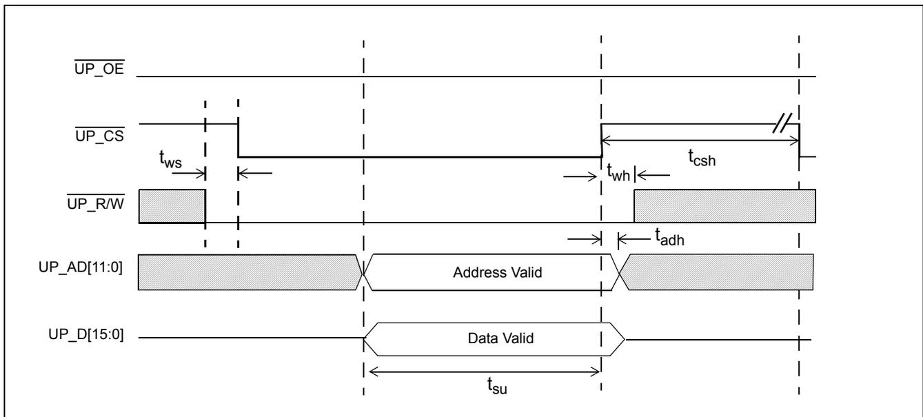
**Figure 25 - CPU Interface Motorola Timing - Write Access**
