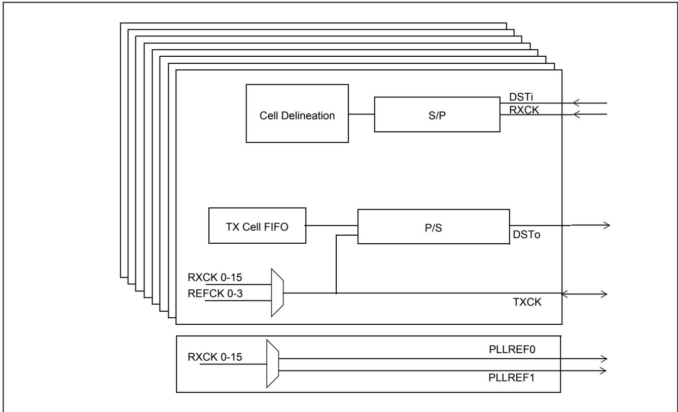
Figure 11 - TXCK Output Pin Source Options
