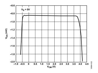
Figure 31. Vos vs. Common-Mode Voltage
