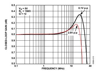
Figure 8. 0.1 dB Flatness Response for Various Output Voltages
