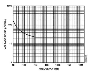
Figure 28. Voltage Noise vs. Frequency
