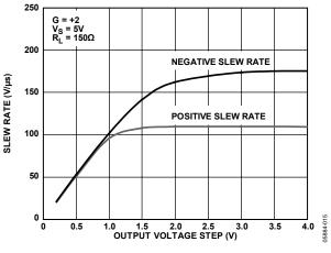
Figure 13. Slew Rate vs. Output Voltage
