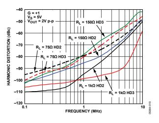
*Figure 20. Harmonic Distortion vs. Frequency*
