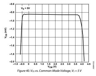
For signals approaching the minus supply and inverting gain and high positive gain configurations, the headroom limit is the output stage. The ADA4853-1 uses a common emitter output stage. This output stage maximizes the available output range, limited by the saturation voltage of the output transistors. The saturation voltage increases with the drive current that the output transistor is required to supply due to the output transistor's collector resistance.
