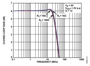
Figure 10. Large Signal Frequency Response for Various Loads
