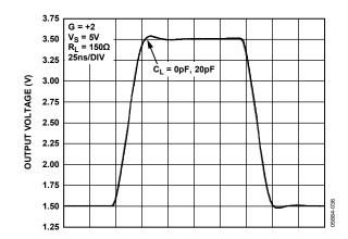
Figure 25. Large Signal Pulse Response for Various Capacitive Loads
