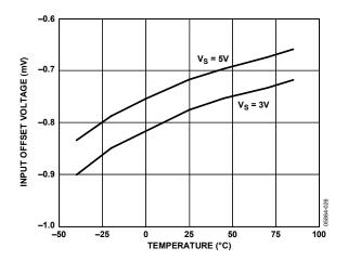
Figure 33. Input Offset Voltage vs. Temperature
