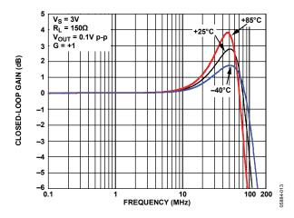
Figure 11. Small Signal Frequency Response for Various Temperatures
