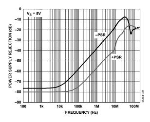
Figure 16. Power Supply Rejection vs. Frequency
