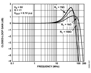
Figure 5. Small Signal Frequency Response for Various Loads
