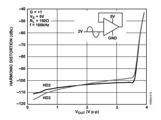
Figure 21. Harmonic Distortion for Various Output Voltages
