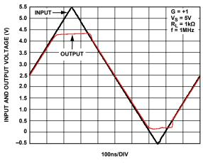
Figure 27. Input Overdrive Recovery
