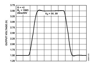
Figure 24. Large Signal Pulse Response for Various Supplies
