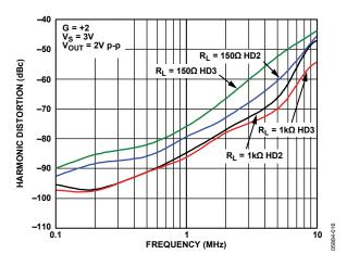
Figure 18. Harmonic Distortion vs. Frequency
