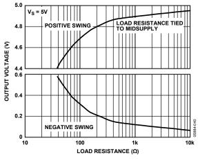
Figure 36. Output Swing vs. Load Resistance
