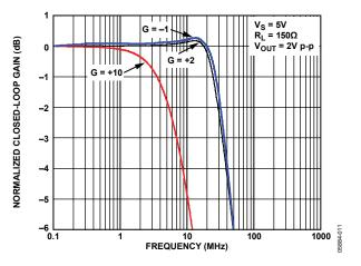
Figure 9. Large Signal Frequency Response for Various Gains
