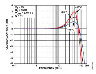
Figure 12. Small Signal Frequency Response for Various Temperatures
