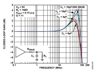
Figure 7. Small Signal Frequency Response for Various Capacitive Loads
