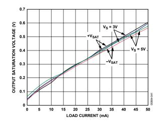
Figure 37. Output Saturation Voltage vs. Load Current
