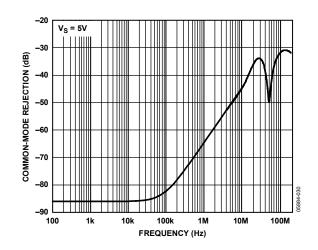
Figure 15. Common-Mode Rejection vs. Frequency
