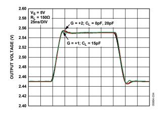
Figure 23. Small Signal Pulse Response for Various Capacitive Loads
