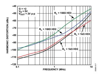
Figure 19. Harmonic Distortion vs. Frequency
