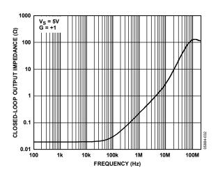
Figure 17. Output Impedance vs. Frequency Enabled
