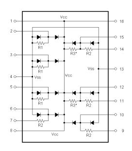
$\begin{array}{l} R1 = 75\Omega, R2 = 33\Omega \\ R3 = 2.2K\Omega \mbox{ (for PACVGA100 only)} \end{array}$
