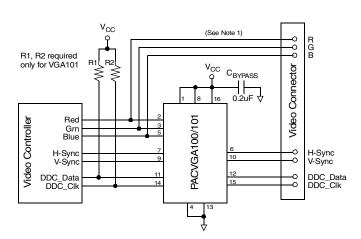
Note 1: For best ESD protection, minimize R/G/B trace lengths between the PACVGA100/101 device and the video connector.
