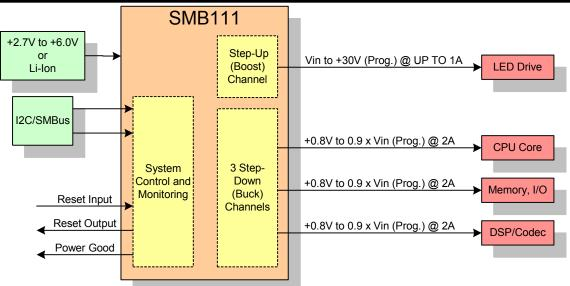
Figure 1: Applications schematic featuring the SMB111 four-channel, programmable DC-DC controller Note: This is an applications example only. Some pins, components and values are not shown.
