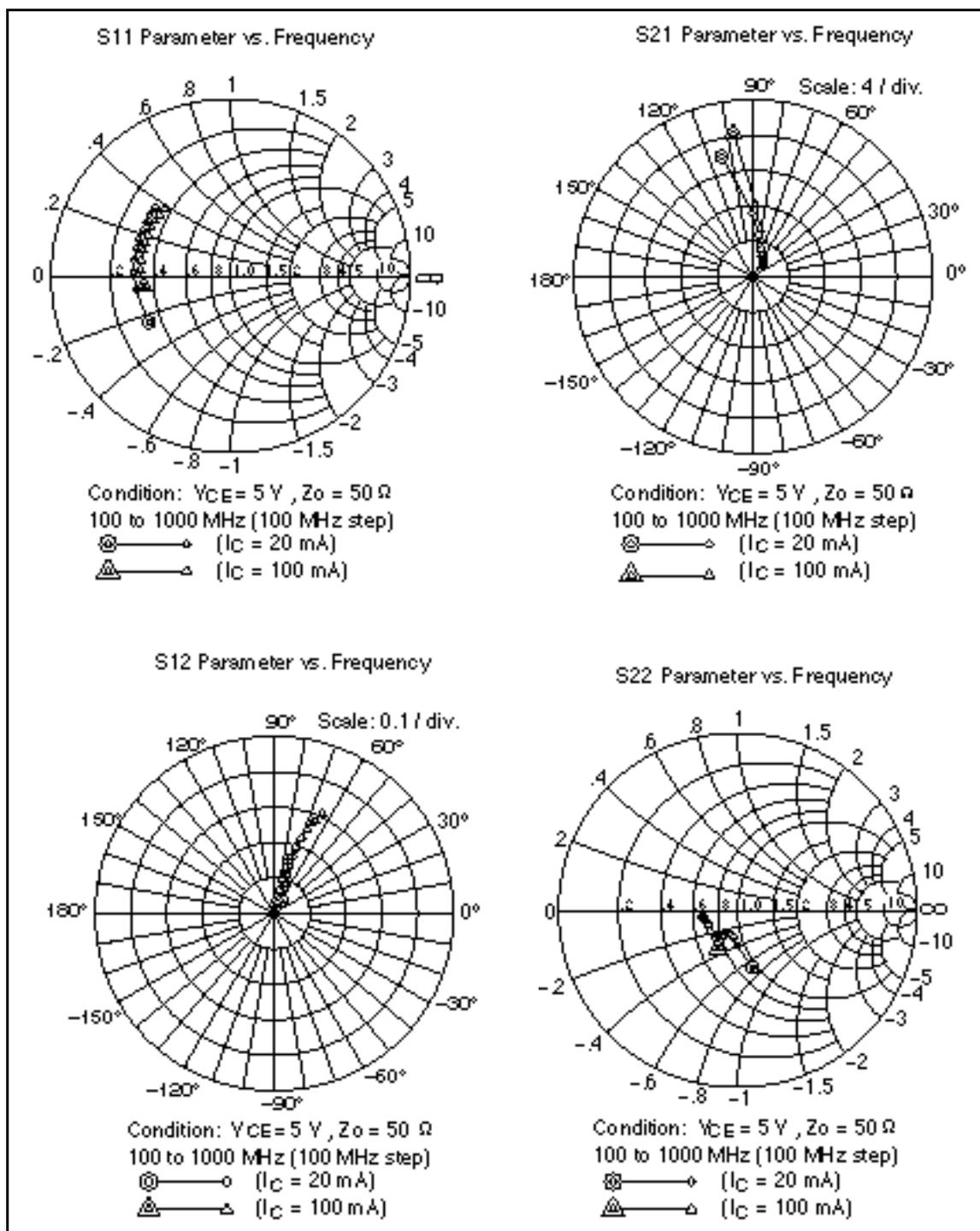
**S Parameter** ( $V_{CE} = 5 \text{ V}$ ,  $I_C = 20 \text{ mA}$ ,  $Z_O = 50 \Omega$ , Emitter Common)
