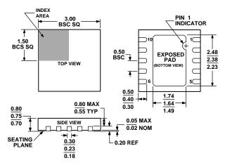
Figure 43. . 10-Lead Lead Frame Chip Scale Package (CP-10-9) Dimensions shown in millimeters
