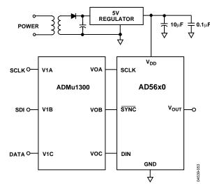
Figure 42. AD5663R with a Galvanically Isolated Interface
