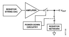
Figure 35. Output Stage During Power-Down
