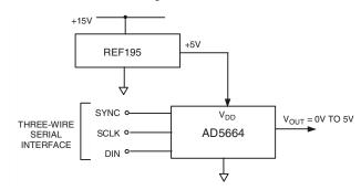
Figure 40. REF195 as Power Supply to the AD5624R/AD5644R/AD5664
