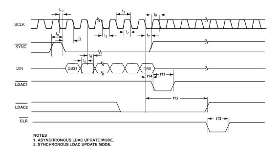
Figure 2. Serial Write Operation
