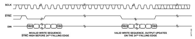
Figure 37 SYNC Interrupt Facility
