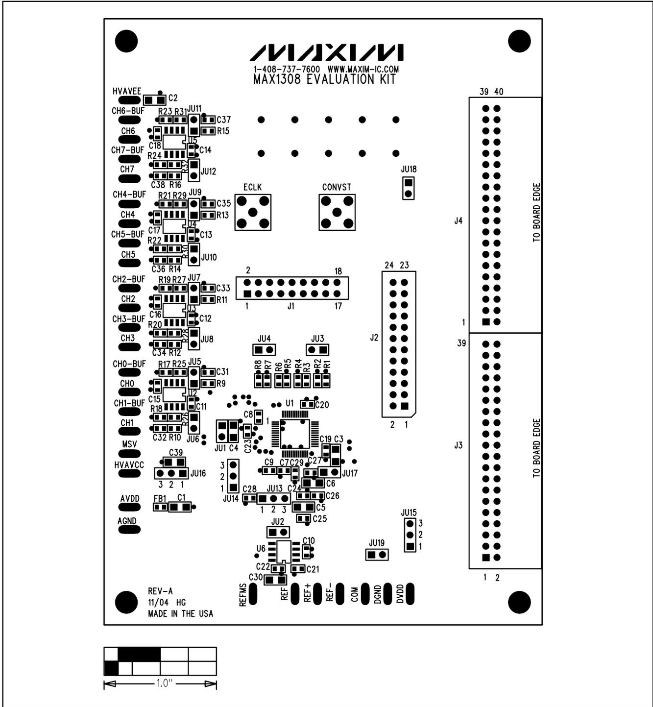
Figure 7. MAX1308 EV Kit Component Placement Guide—Component Side
