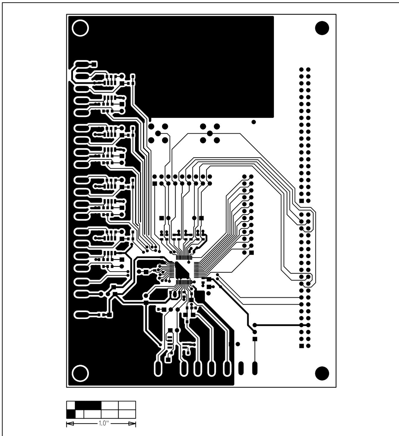
Figure 8. MAX1308 EV Kit PC Board Layout—Component Side
