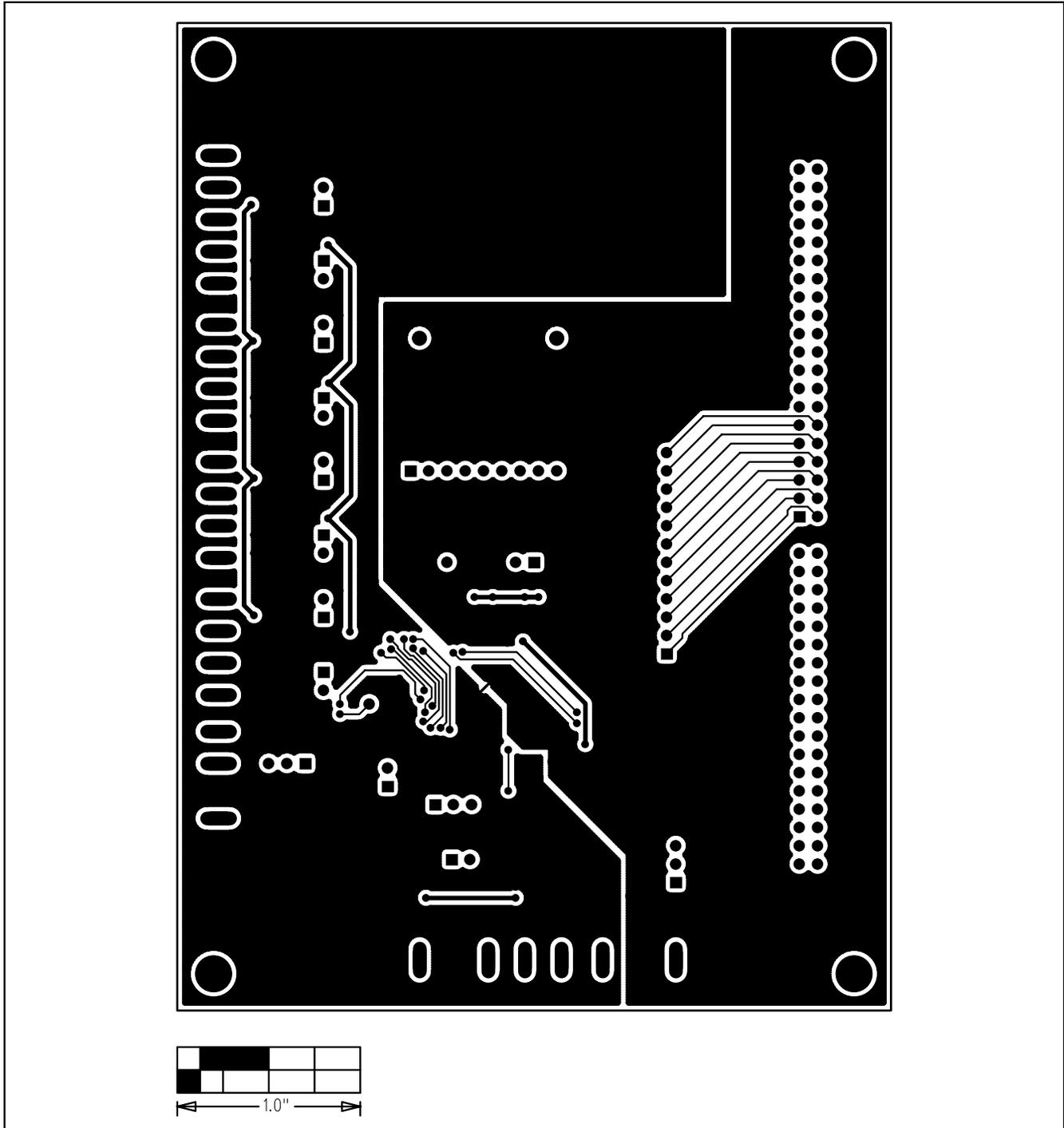
Figure 9. MAX1308 EV Kit PC Board Layout—Solder Side
