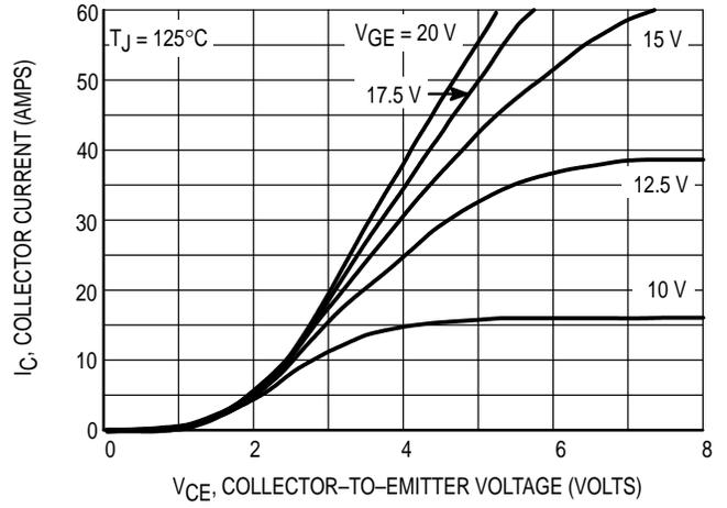
Figure 2. Output Characteristics
