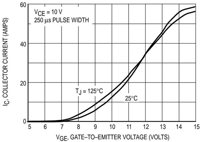
Figure 3. Transfer Characteristics
