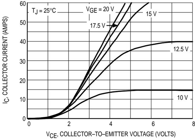
Figure 1. Output Characteristics
