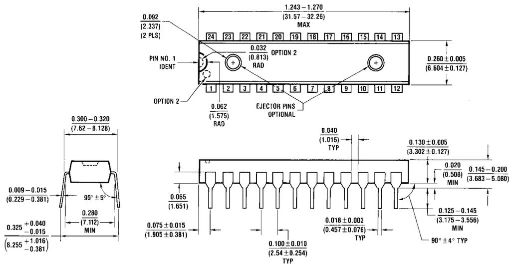
**24-Lead Plastic Dual-In-Line Package (PDIP), JEDEC MS-100, 0.300 Wide
