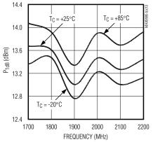
INPUT P1dB vs. RF FREQUENCY
