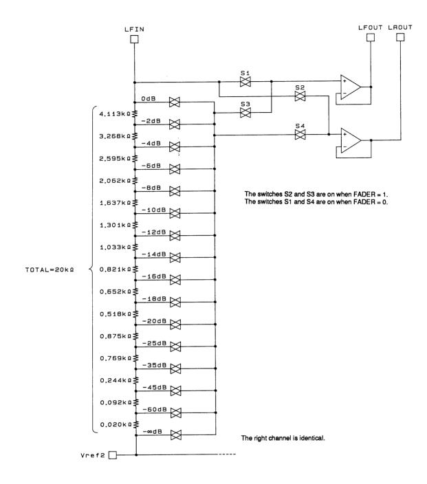
If data setting the main volume control 1-dB step to  $-\infty$  is sent to the LSI, the S1 and S2 switches will be opened and the S3 and S4 switches will be turned on (closed).
