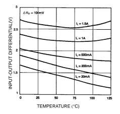
Figure 3. Dropout Voltage
