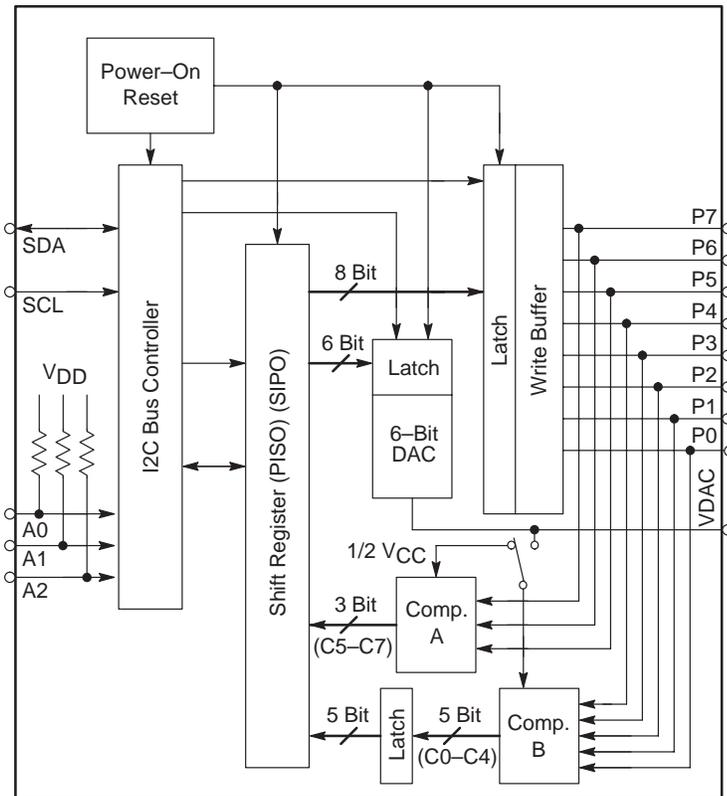
NOTE: Internal Power On Reset sets P0 ~ P7 low, sets VDAC to 1/80 V<sub>DD</sub> and selects 1/2 V<sub>DD</sub> for Comparator "B" threshold.
