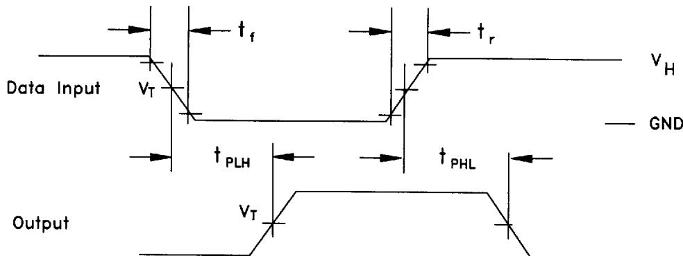
Input and output threshold voltage:
