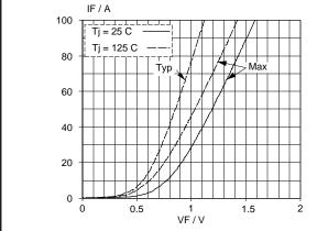
Fig.3. Typical and maximum forward characteristic per diode;  $I_F = f(V_F)$ ; parameter  $T_i$
