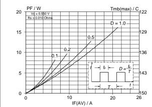
Fig.1. Maximum forward dissipation  $P_F = f(I_{F(AV)})$  per diode; square current waveform where  $I_{F(AV)} = I_{F(RMS)} \times \sqrt{D}$ .
