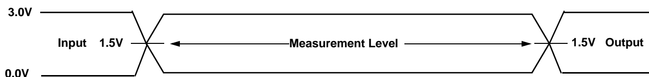
Figure 15. Input Waveforms and Measurement Levels
